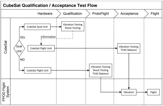
Figure 8: CubeSat General Testing Flow Diagram
