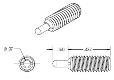
Figure 5: Custom Spec Spring Plunger (Separation Spring)
