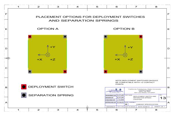
Figure 7: Deployment Switches and Separation Spring Locations
