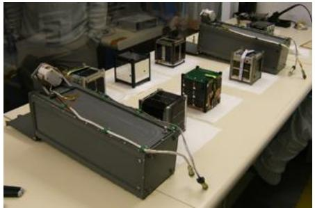
Figure 1: Six CubeSats and their deployment systems.
