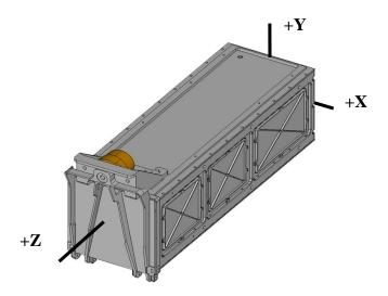
Figure 4: PPOD Coordinate System
